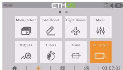
Choose the INT MODULE. Then turn ON INTERNAL RF, select the OUTSIDE or INSIDE ANTENNA. Set the Mode for Horus X12S-ISRМ internal RF corresponding to your receiver (ACCESS, ACCST D16).
