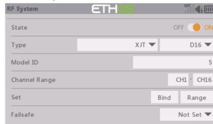
The external RF module can be powered on or off by software. The setup process is the same as that for the internal RF. External modules should be closed when not in use.
